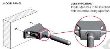
Recommended fixing pan head screw type - head Ø 5 mm max.
