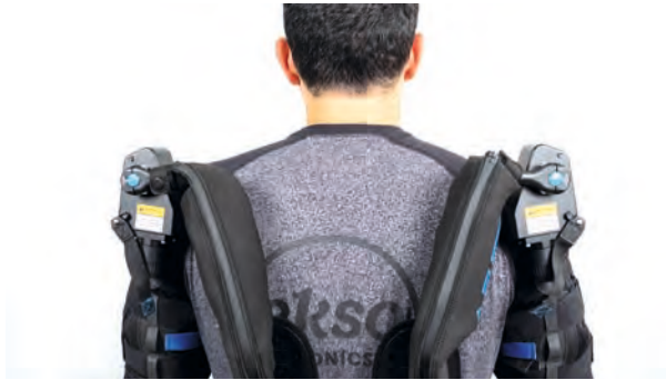
Figure 10: Proper Ekso EVO Actuator Height Alignment
