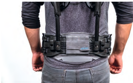
Figure 11: Ekso EVO in narrow position
