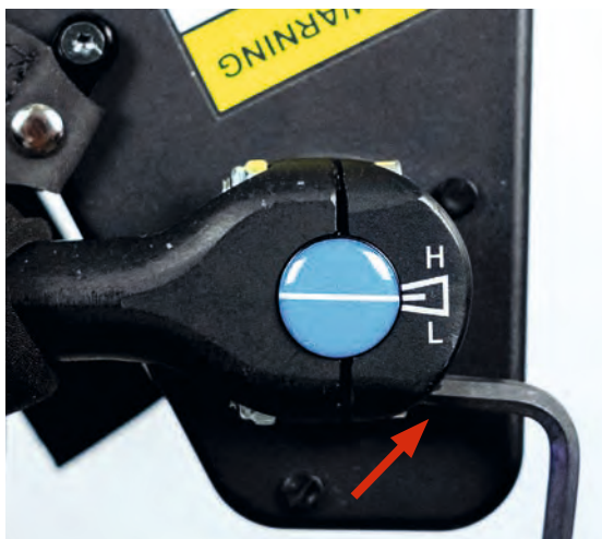
Figure 19: Loosening End Link Screw
