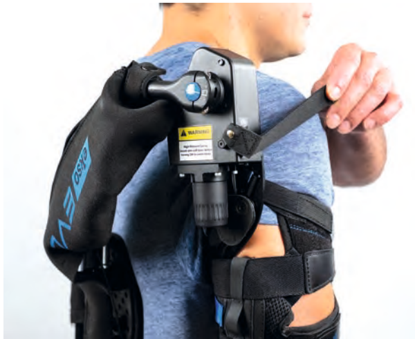
Figure 16: Turning Ekso EVO On
