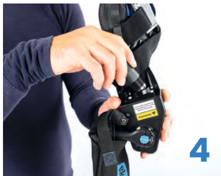
Figure 17: Installing Actuator Springs
